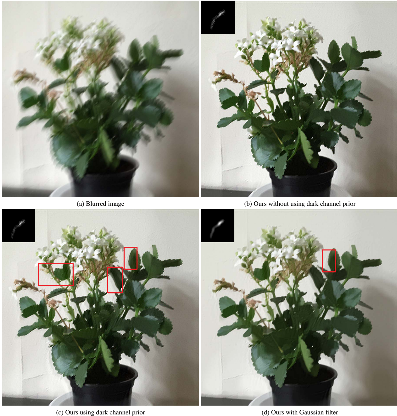
Figure 10. The proposed dark channel prior is sensitive to the Gaussian noise. Since the noise will change the minimum intensity value of an image patch, the deblurred image generated with dark channel prior still contains blur effect as shown in the parts in red boxes in (c), while the deblurred image generated without using dark channel prior is much clearer. We note that although the kernel estimate looks better after applying Gaussian filter to the blurred input, the final deblurred image looks over smooth and still contains ringing artifacts as shown in the red box in (d) due to influence of the filter.
