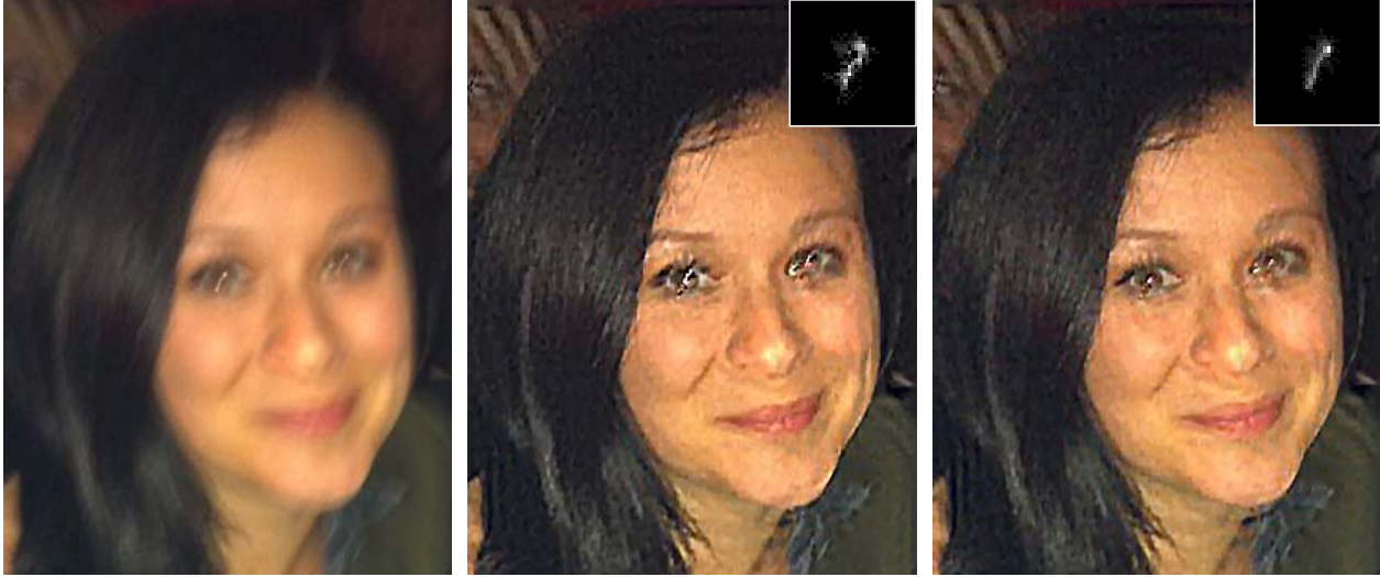
(a) Blurred images (b) Ours without using dark channel prior (c) Ours using dark channel prior
