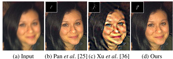
Figure 10. Comparisons on blurred face images. Our method compares favorably with [25], which uses a face dataset to explore face structures for deblurring face images.
